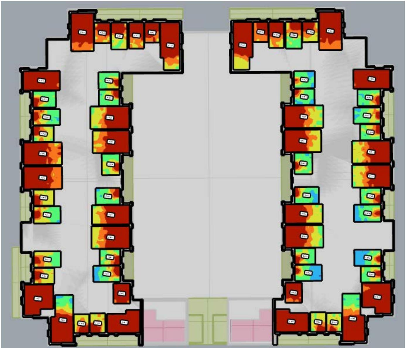
Figure 31: Blocks A & B Third Floor, showing rooms assessed with false colour plan for the ADF. The scale is from 0-5%.
