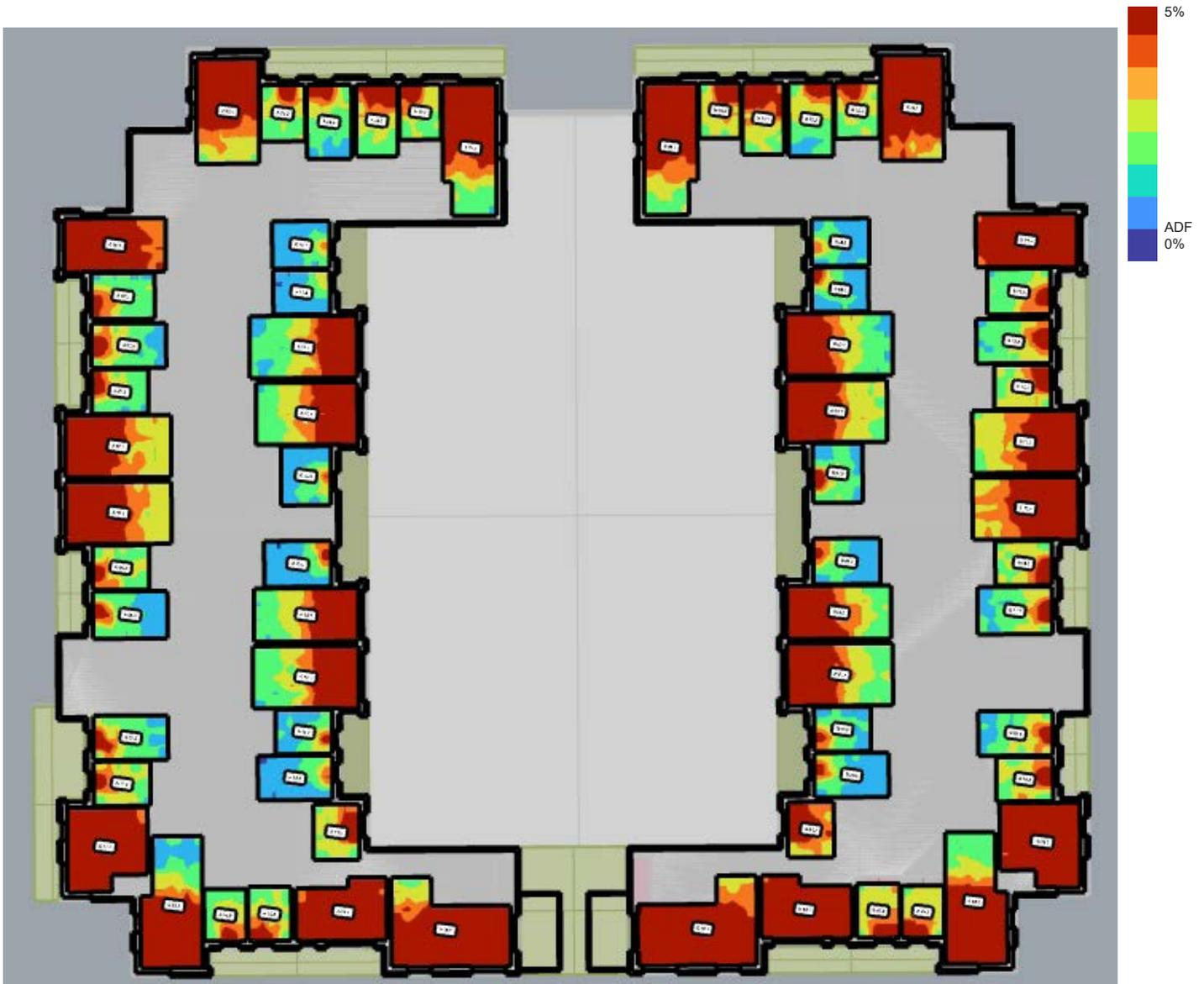
Figure 29: Blocks A & B First Floor, showing rooms assessed with false colour plan for the ADF. The scale is from 0-5%.
