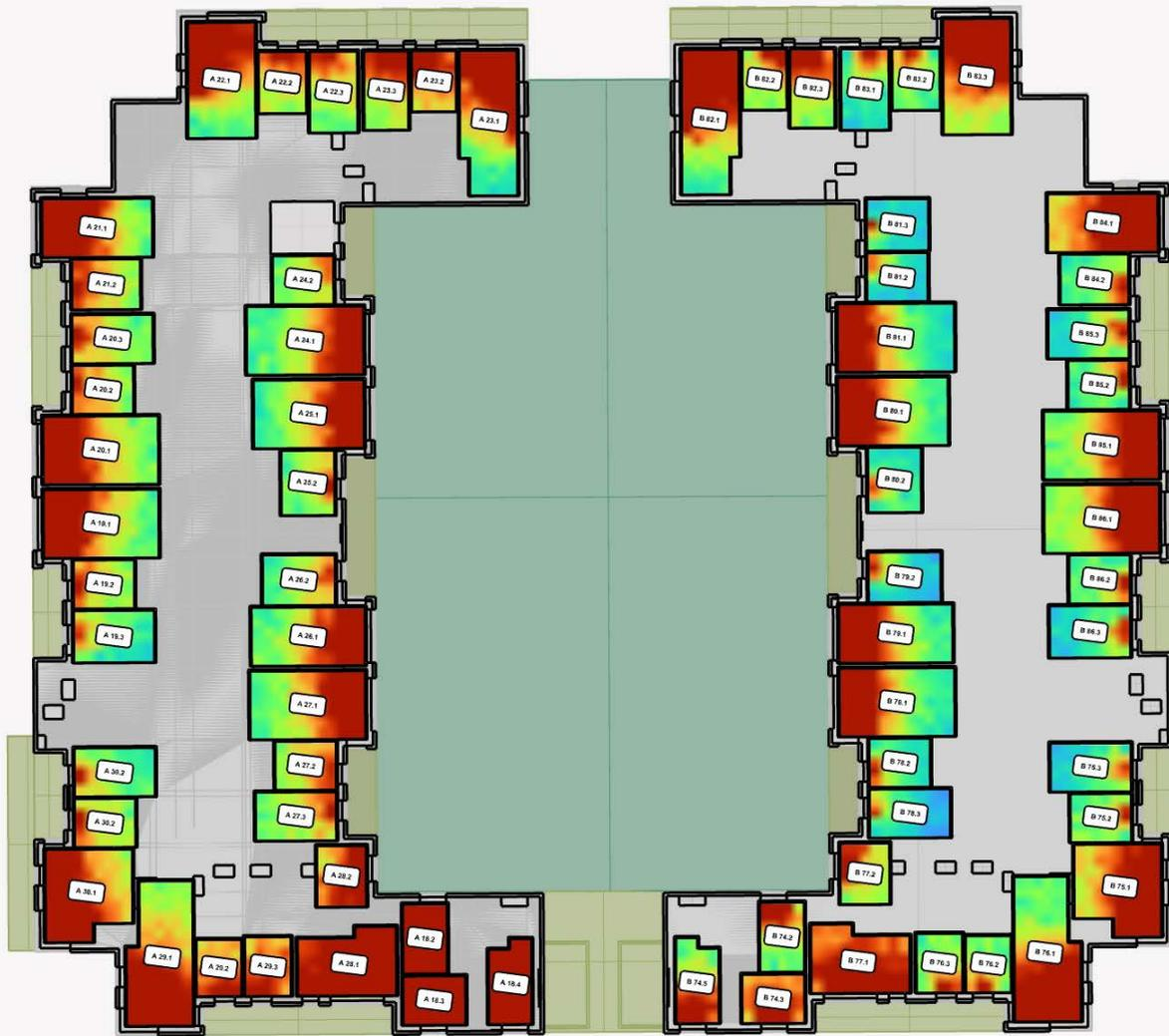
Figure 30: Blocks A & B Second Floor, showing rooms assessed with false colour plan for the ADF. The scale is from 0-5%.
