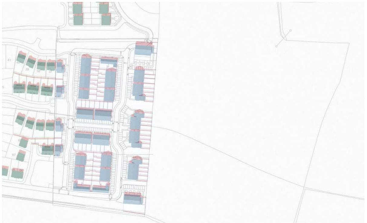
**Figure 17: Shadow diagrams 21 June 14:00 GMT+1 (DST)**
