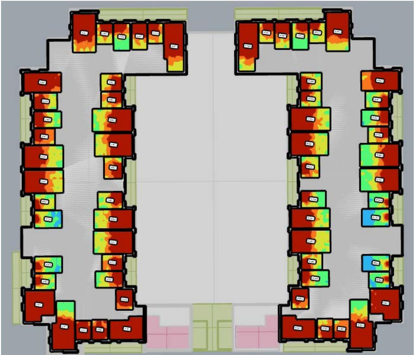
Figure 32: Blocks A & B Fourth Floor, showing rooms assessed with false colour plan for the ADF. The scale is from 0-5%.
